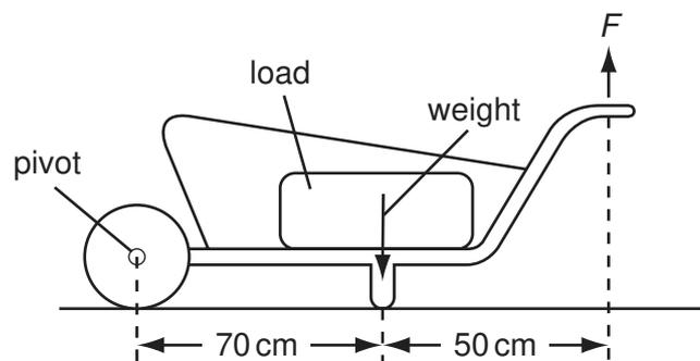
What is the size of force  $F$  needed just to lift the loaded wheelbarrow?
