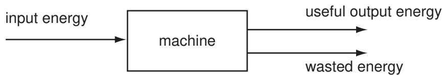
The machine is 50% efficient.
